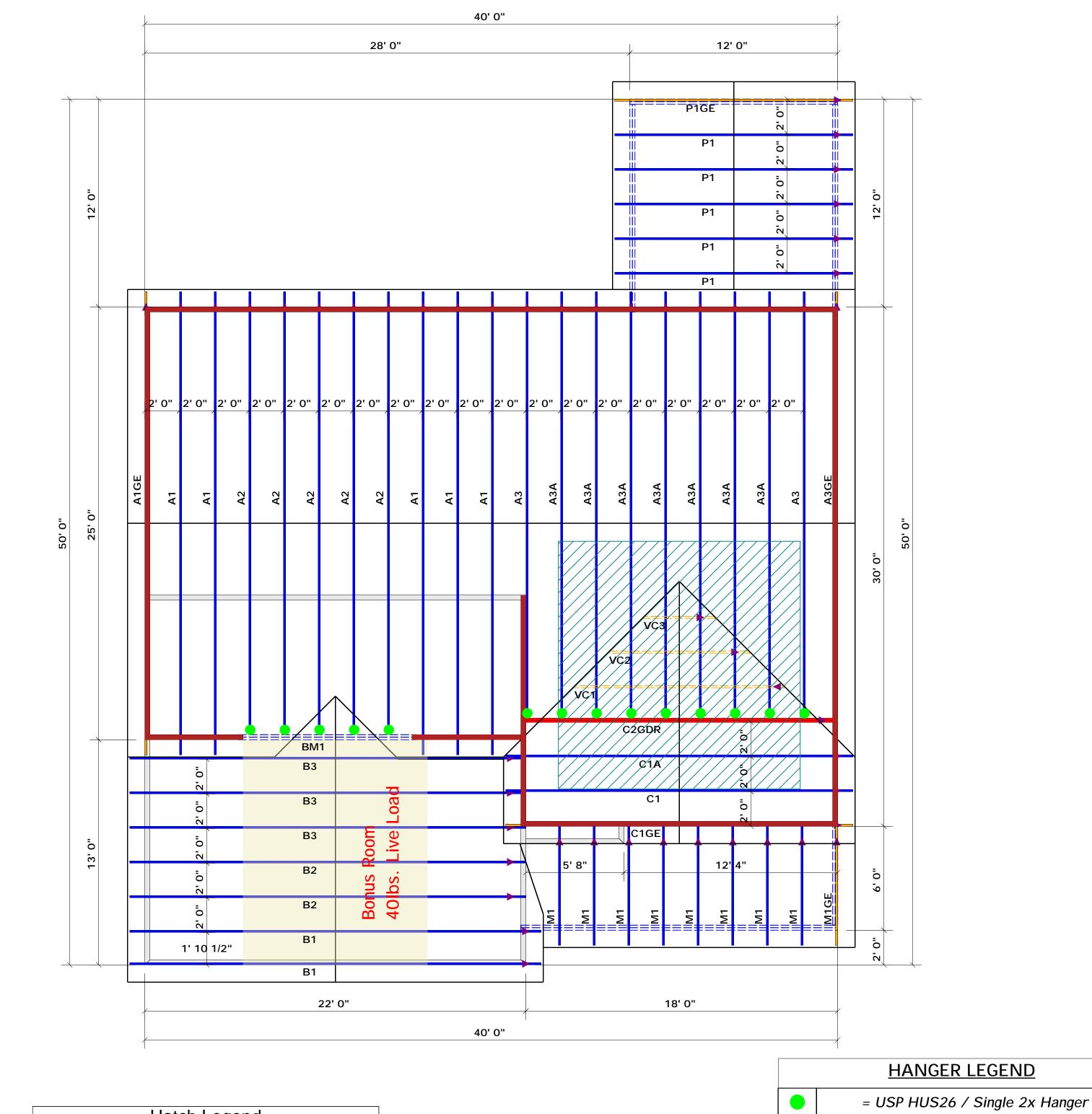
▲ = Denotes Left End of Truss(Reference Engineered Truss Drawing)Do Not Erect Trusses Backwards
