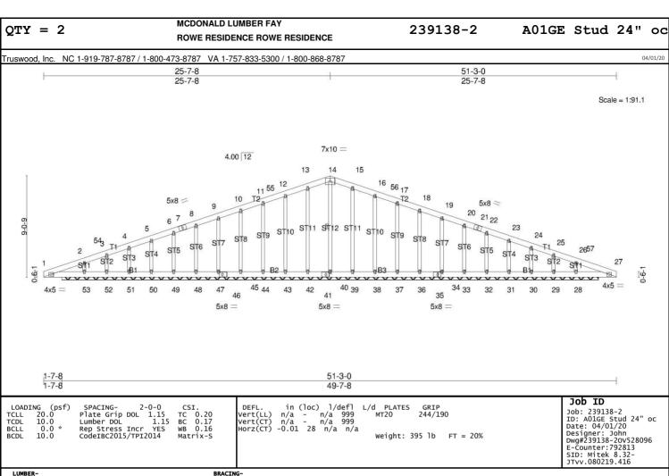
LUMBER-TOP CHORD 2x6 SP No.2 BOT CHORD 2x6 SP No.2 OTHERS 2x4 SP No.3 BRACING TOP CHORD BOT CHORD -Structural wood sheathing directly applied or 10-0-0 oc purlins. Rigid ceiling directly applied or 6-0-0 oc bracing. 1 Row at midpt 14-40
