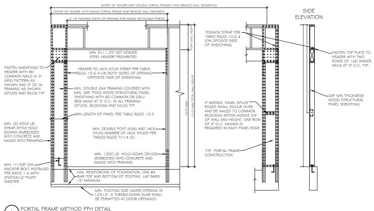
AS A SUBSTITUTE FOR THE USP STADI4 HOLD-DOWN STRAPS LOCATED ON EACH SIDE OF THE GARAGE DOO DPENING, SIMPSON HDQ8-SD53 (OR USP PHD8) HOLD-DOWNS MAY BE INSTALLED. THE SIMPSON HDQ8-SD53 (US PHD8) HOLD-DOWNS MAY BE INSTALLED WITH 7/8" THREADED ROD AND SHOULD BE EMBEDDED A MINIMUM OF 8
