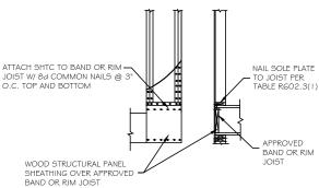
WOOD STRUCTURAL PANEL ATTACH SHTC TO BAND OR RIM -HEATHING CONTINUOUS OVER JOIST W/ 8d COMMON NAILS @ O.C. TOP AND BOTTOM NAIL SOLE PLATE TO JOIST PER TABLE R602.3(1) WOOD STRUCTURAL PANEL HEATHING OVER APPROVED BAND OVER RAISED WOOD FLOOR - OVERLAP OPTION
