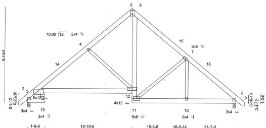
1-9-8 Plate Offsets (X,Y)--[2:0-0-0,0-0-4], [3:0-6-0,0-1-3], [5:0-3-9,0-0-0], [5:0-4-5,0-1-12], [6:0-2-5,0-2-12] LOADING (psf) SPACING-2-0-0 CSI. DEFL in (loc) I/defl L/d **PLATES** GRIP TCLL 20.0 Plate Grip DOL 1.15 TC 0.39 Vert(LL) -0.123-12 >999 360 MT20 244/190 TCDL 10.0 Lumber DOL BC 1.15 0.42 Vert(CT) -0.28 3-12 >897 240 BCLL 0.0 Rep Stress Incr YES WB 0.35 Horz(CT) 0.14 8 n/a n/a BCDL 10.0 Code IRC2015/TPI2014 Matrix-S Wind(LL) 0.06 3-12 >999 240 Weight: 172 lb FT = 20%
