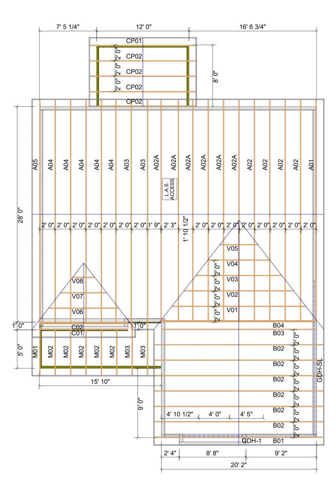
THE SUGGESTED TRUSS HANGERS, CONNECTIONS AND TIE-DOWNS FOR GRAVITY, UPLIFT AND LATERAL LOADS, MUST BE REVIEWED BY THE BUILDING DESIGNER OR ENGINEER OF RECORD. PER ANSI/TPI 1-2002, ALL "TRUSS TO WALL" AND "TRUSS TO BEAM" CONNECTIONS ARE THE RESPONSIBILITY OF THE BUILDING DESIGNER. ALL TRUSS TO TRUSS" CONNECTIONS ARE THE RESPONSIBILITY OF THE TRUSS DESIGNER/ MANUFACTURER
