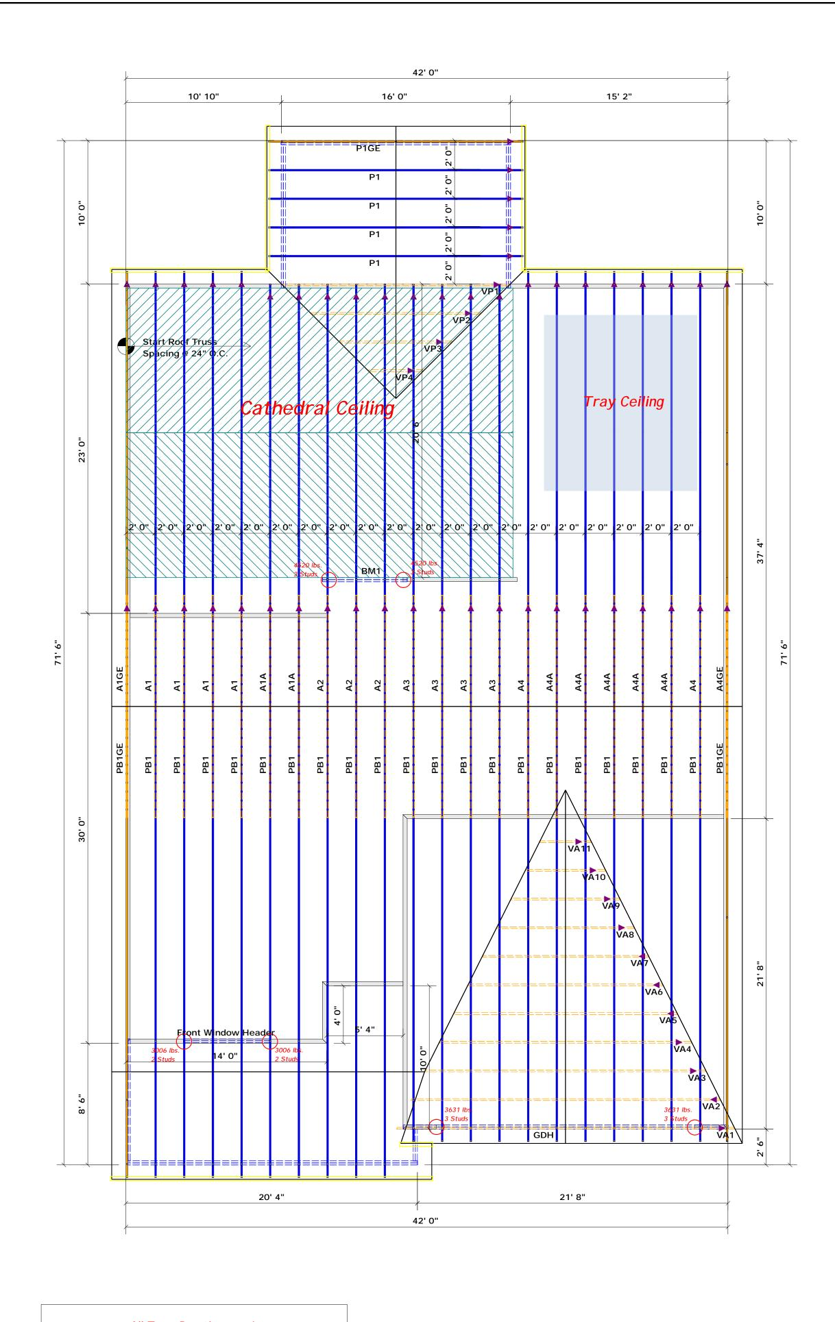
▲ = Denotes Left End of Truss(Reference Engineered Truss Drawing)Do Not Erect Trusses Backwards
