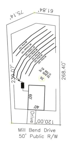
If plumbing is not sufficient a pump and tank may be required to septic drain field.
