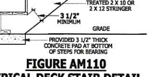
FIGURE AM110 TYPICAL DECK STAIR DETAIL SCALE 3/4" = 1'-0"
