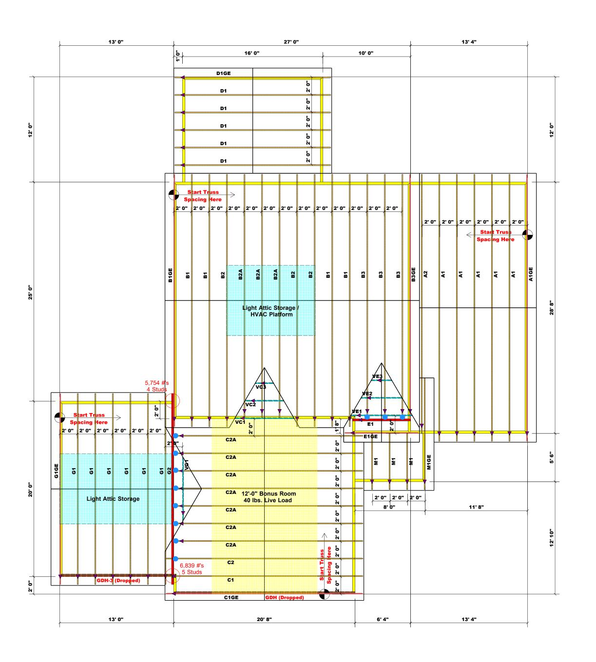
▲= Denotes Left End of Truss (Reference Engineered Truss Drawing)
