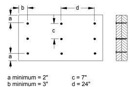
Connectors are: 3-1/4 in. Pneumatic Gun Nails
