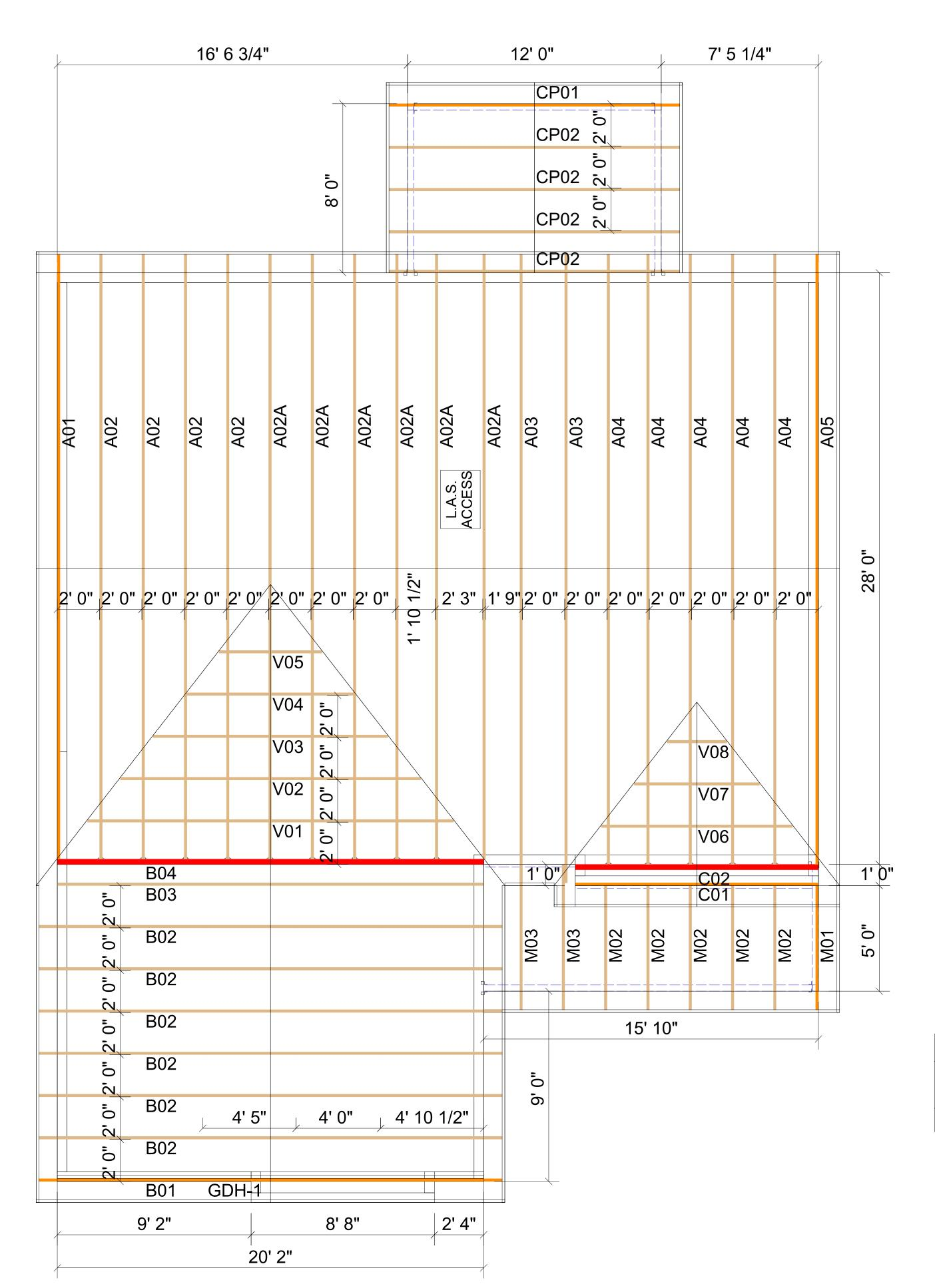
THE SUGGESTED TRUSS HANGERS, CONNECTIONS AND TIE-DOWNS FOR GRAVITY, UPLIFT AND LATERAL LOADS, MUST BE REVIEWED BY THE BUILDING DESIGNER OR ENGINEER OF RECORD. PER ANSI/TPI 1-2002, ALL "TRUSS TO WALL" AND "TRUSS TO BEAM" CONNECTIONS ARE THE RESPONSIBILITY OF THE BUILDING DESIGNER. ALL "TRUSS TO TRUSS" CONNECTIONS ARE THE RESPONSIBILTY OF THE TRUSS DESIGNER/ MANUFACTURER
