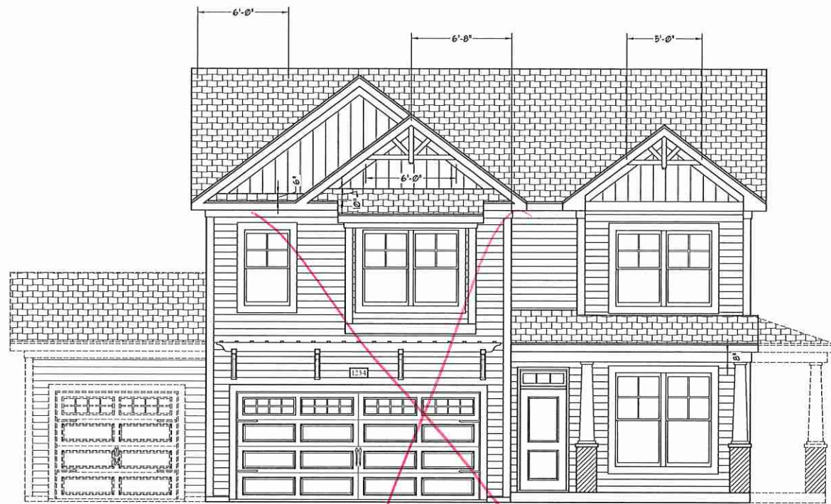
FRONT ELEVATION-B-1 SCALE: 1/4" = 1'-0"
