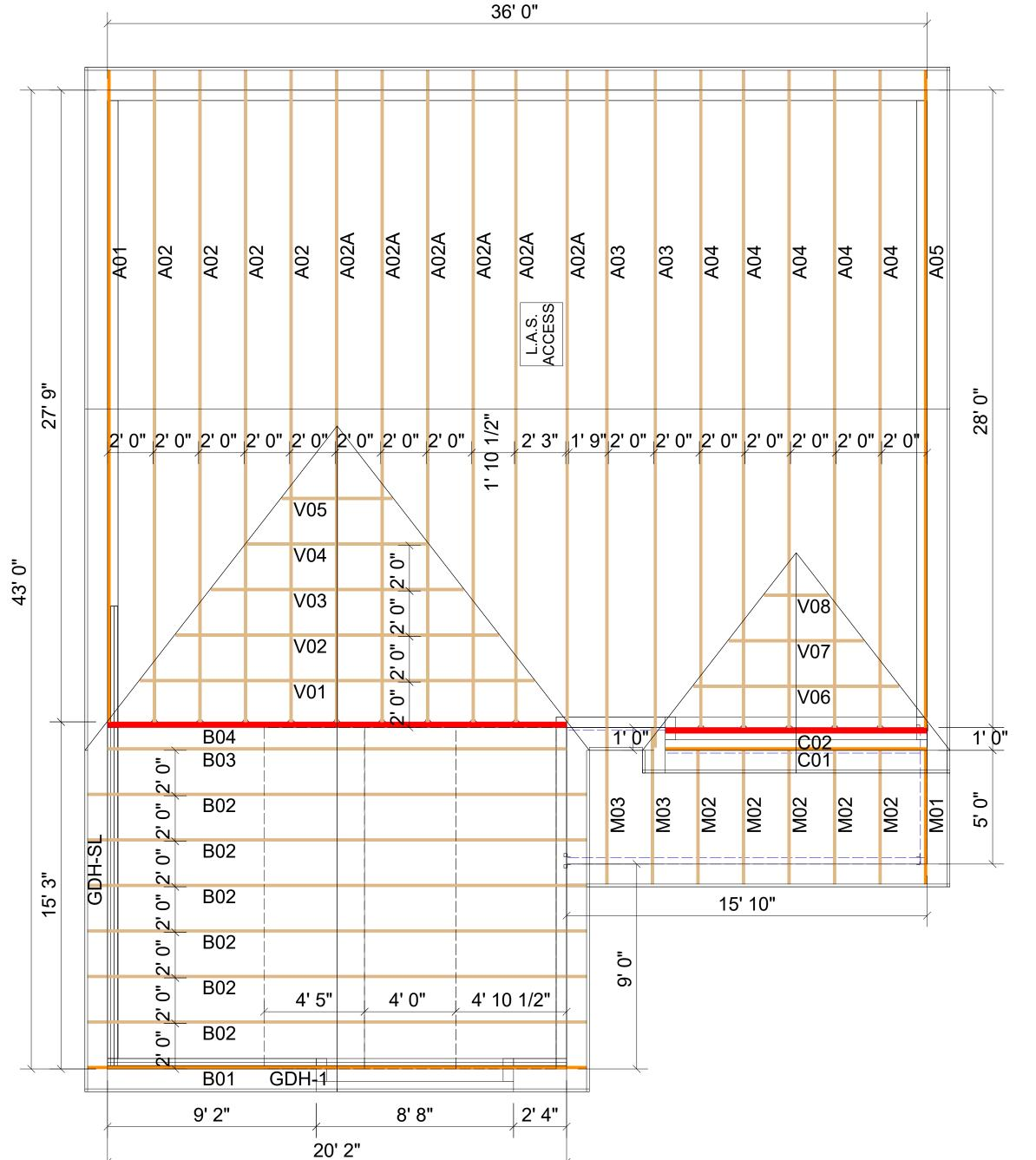
THE SUGGESTED TRUSS HANGERS, CONNECTIONS AND TIE-DOWNS FOR GRAVITY, UPLIFT AND LATERAL LOADS, MUST BE REVIEWED BY THE BUILDING DESIGNER OR ENGINEER OF RECORD. PER ANSI/TPI 1-2002, ALL "TRUSS TO WALL" AND "TRUSS TO BEAM" CONNECTIONS ARE THE RESPONSIBILITY OF THE BUILDING DESIGNER. ALL "TRUSS TO TRUSS" CONNECTIONS ARE THE RESPONSIBILTY OF THE TRUSS DESIGNER/ MANUFACTURER
