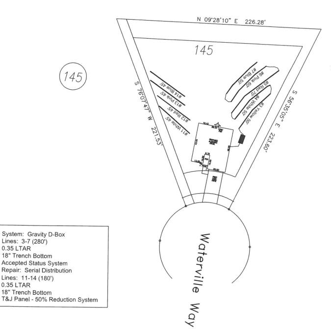
System: Gravity D-Box Lines: 3-7 (280') 0.35 LTAR 18" Trench Bottom Accepted Status System Repair: Serial Distribution Lines: 11-14 (180') 0.35 LTAR 18" Trench Bottom
