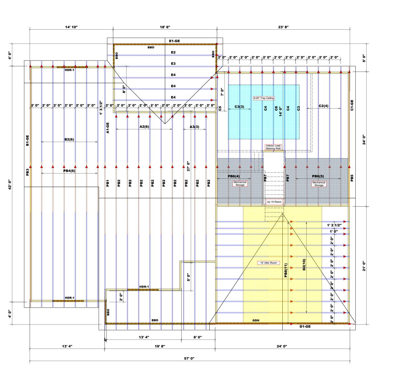
All Truss Reactions are Less than 3,000 lbs. Unless Noted Otherwise. -- Denotes Reaction Greater than 3,000 lbs. Reaction / # of Studs
