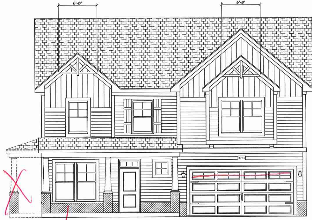
Stone FRONT ELEVATION-B-2 SCALE: 1/4" = 1'-0"
