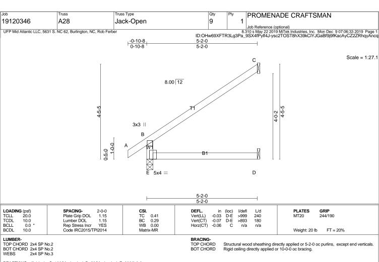
REACTIONS. (lb/size) C=136/Mechanical, D=56/Mechanical, E=266/0-3-8 Max Horz E=140(LC 10)
