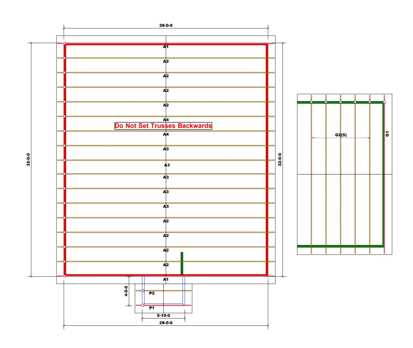
Truss Placement Plan SCALE: NTS
