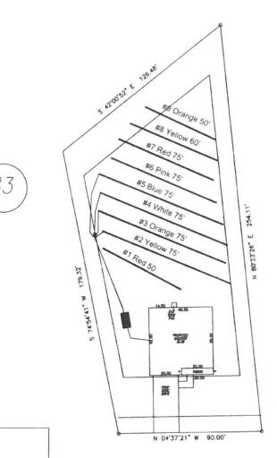
System: Gravity D-Box Lines: 2-5 (300') 0.4 LTAR 20" Trench Bottom Accepted Status System Repair: Pressure Manifold Lines: 1, 6-9 (300')
