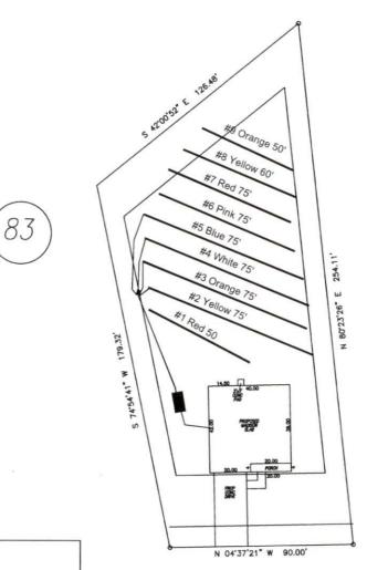
System: Gravity D-Box Lines: 2-5 (300') 0.4 LTAR 20" Trench Bottom Accepted Status System Repair: Pressure Manifold Lines: 1, 6-9 (300') 0.4 LTAR
