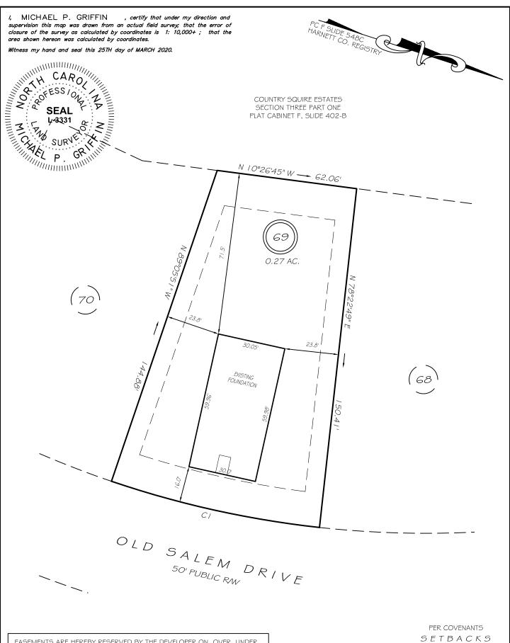
EASEMENTS ARE HEREBY RESERVED BY THE DEVELOPER ON, OVER, UNDER, ABOVE AND THROUGH A STRIP OF LAND TEN FEET IN WIDTH ALONG EACH SIDE LOT LINE AND FIFTEEN FEET IN WIDTH ALONG EACH REAR LOT LINE AND FRONT LOT LINE FOR DRAINAGE, WATER AND SEWAGE INSTALLATION AND MAINTENANCE AND FOR OTHER UTILITY PURPOSES.
