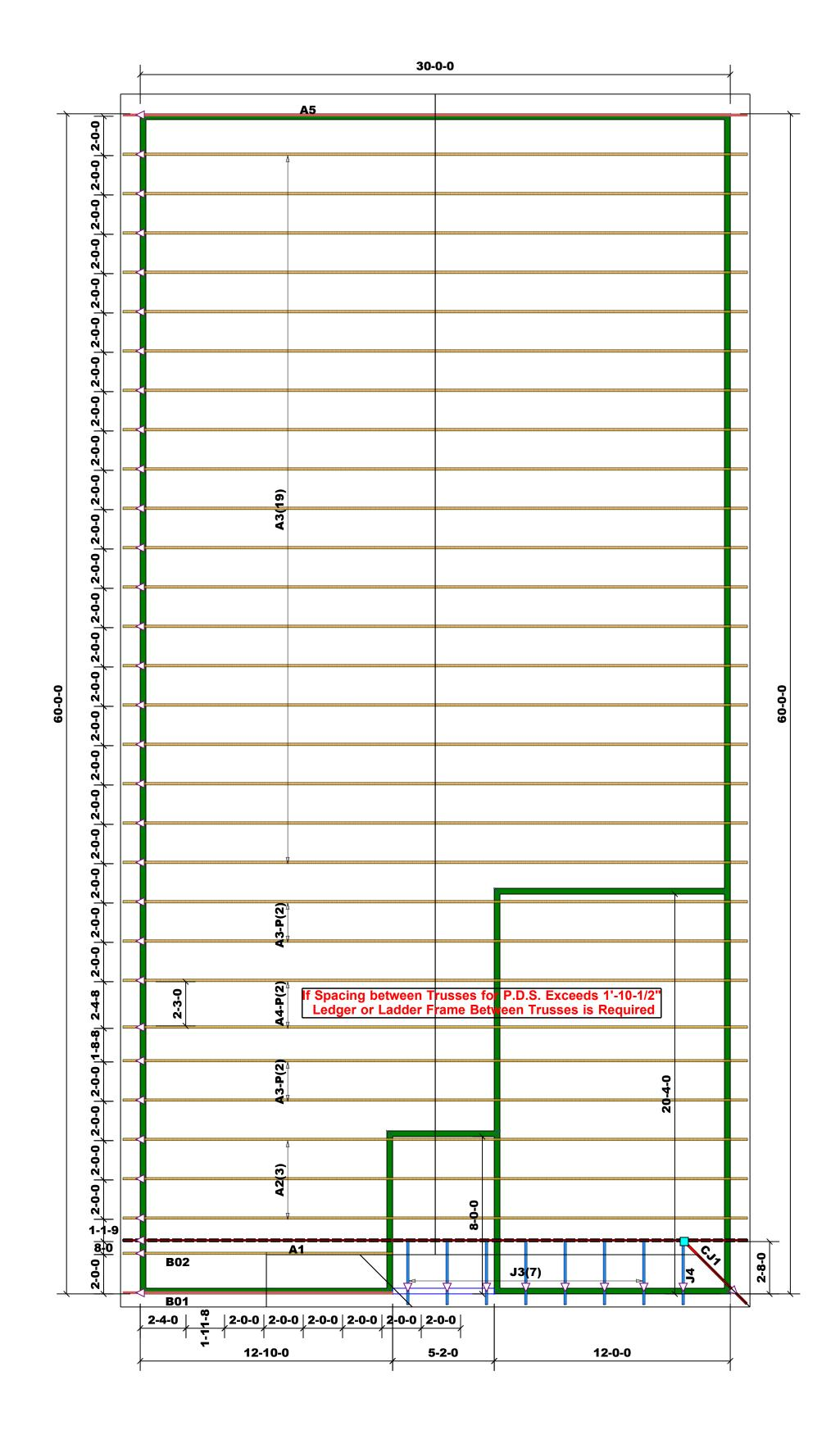
Truss Placement Plan SCALE: NTS
