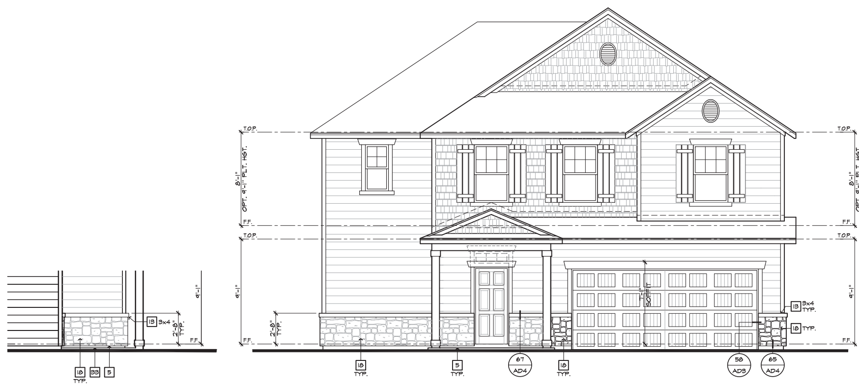
LEFT ELEVATION 'C' W/ OPTIONAL MASONRY AT OPTIONAL 9'-1" PLT. HGT. SCALE 1/4"=1'-0" (22'X34") - 1/8"=1'-0" (11'X17")
