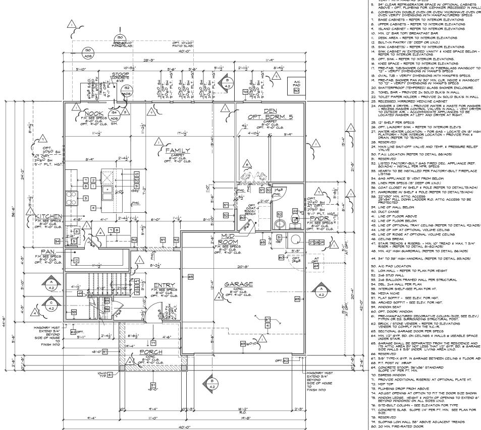
NOTE: NOT ALL KEY NOTES APPLY. SINK - GARBAGE DISPOSAL OPTIONAL - VERIFY DIMENSIONS WITH MANUFACTURERS' SPECS DISHMASHER - PROVIDE AIR GAP - VERIFY SPACING & DIMENSIONS PER MANUFACTURERS' SPECS SLIDE-IN RANGE/OVEN COMBINATION W/ BUILT-IN NON-VENTED HOOD W/LIGHT & FAN. - VERIFY WITH MANUFACTURERS' SPECS
