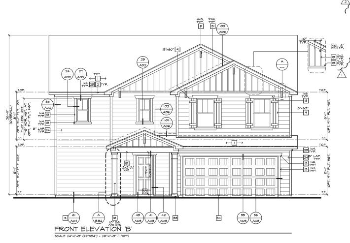
**ELEVATION NOTES** ROOF MATERIAL - REFER TO ROOF NOTES 2. 2X FASCIA/BARGE BOARD WITH FASCIA CAP HOME 12. DECORATIVE TRIM FYPON OR EQ. SEE ELEVATION FOR TYPE 13. TRIM PER SPEC- SEE ELEVATION FOR SIZE
