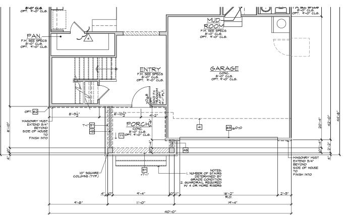
PARTIAL FIRST FLOOR PLAN 'B' AT CRAWL SPACE
