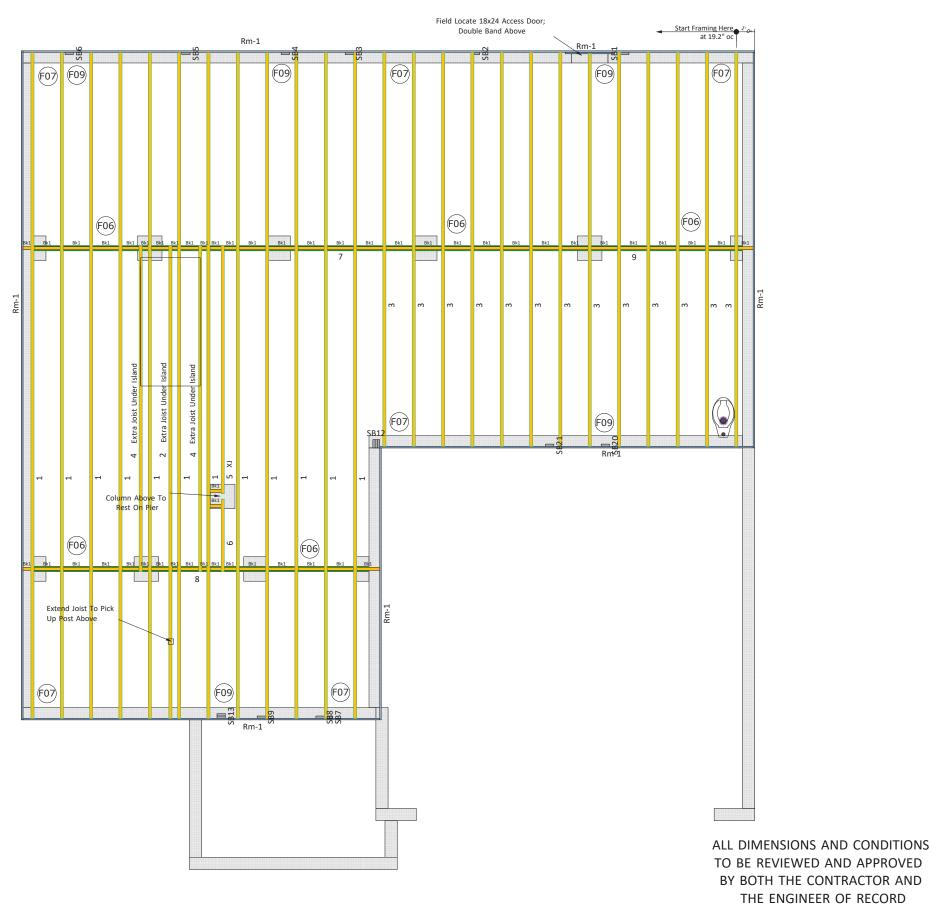
Squash Blocks Required Under The Ends Of All LVL And Point Loads For Load Transfer - See Details
