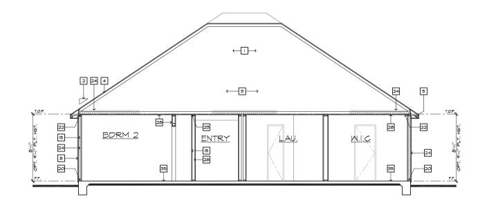
SECTION "A" SCALE |/4"=1'-0" (22"X34") - |/8"=1'-0" (||"X17") AT SLAB-ON-GRADE
