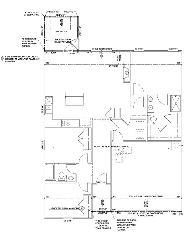
**FIRST FLOOR CEILING FRAMING PLAN - 'B'**
