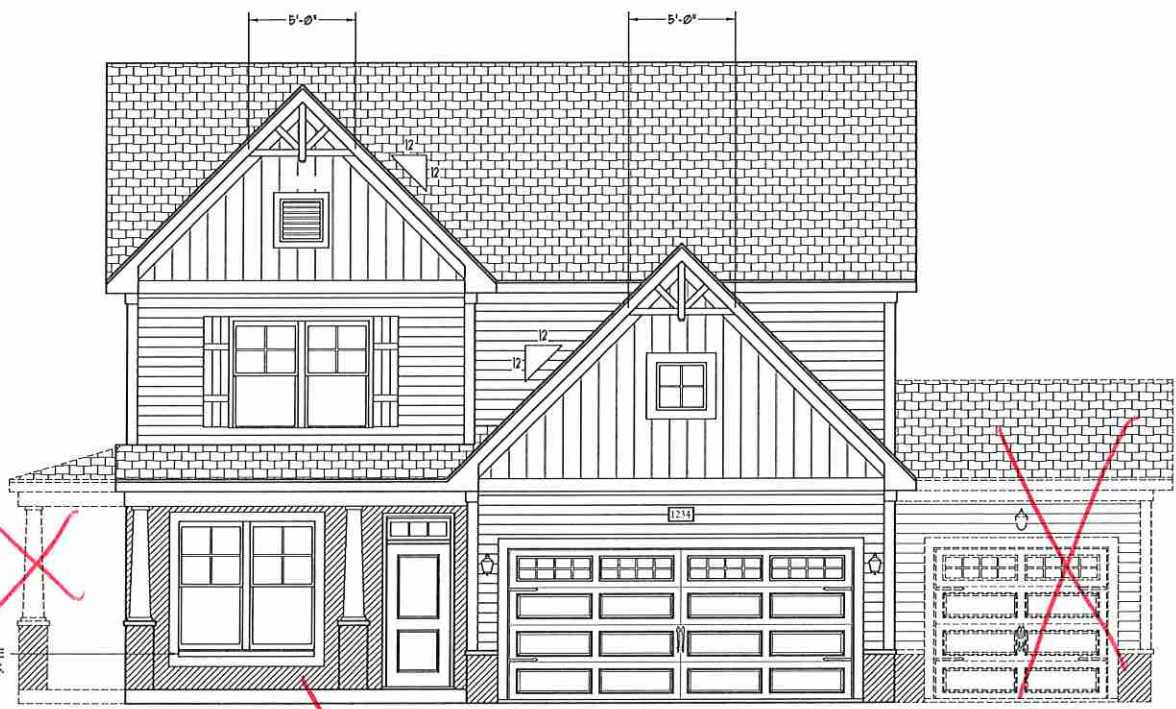
FRONT ELEVATION-B-2 SCALE: 1/4" = 1'-0"
