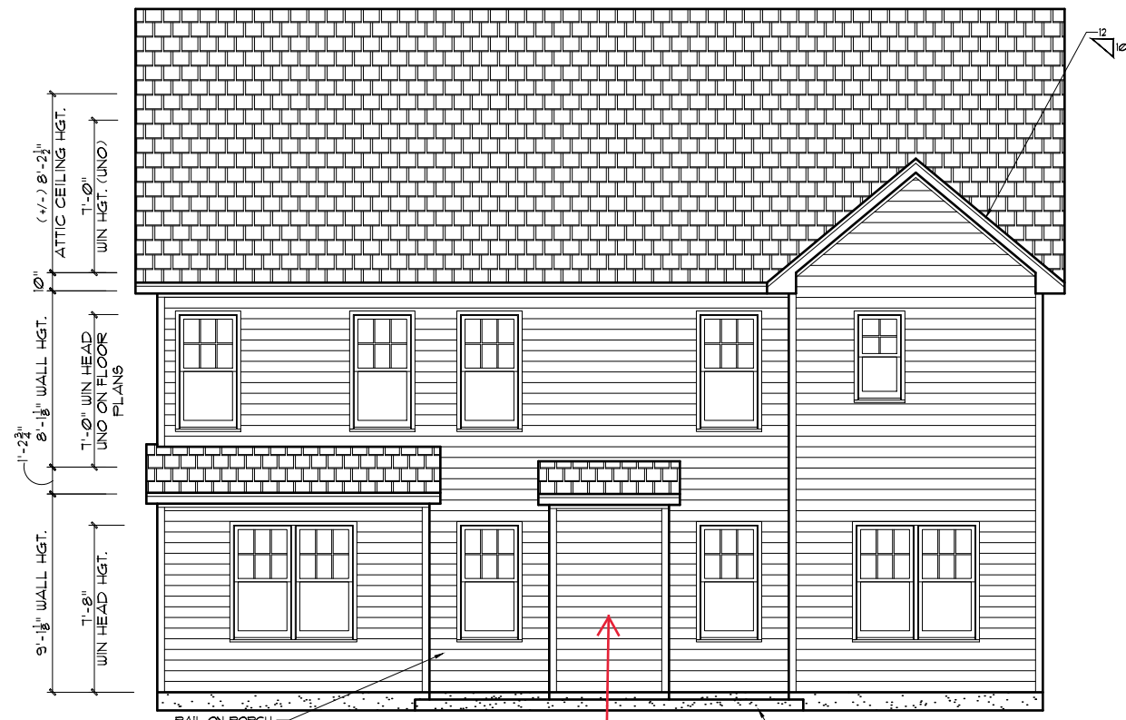
REAR ELEVATION - CRAFTSMAN 22x34 PRINTS SCALE: 1/4"=1'-0" 11x17 PRINTS SCALE: 1/8"=1'-0" STEPS DOWN TO GRADE (NUMBER OF RISERS PER SITE CONDITIONS).
