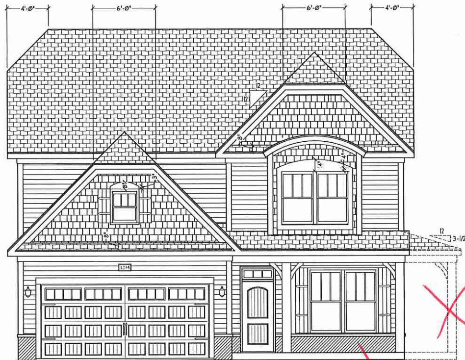
FRONT ELEVATION-C-2 SCALE: 1/4" = 1'-0"
