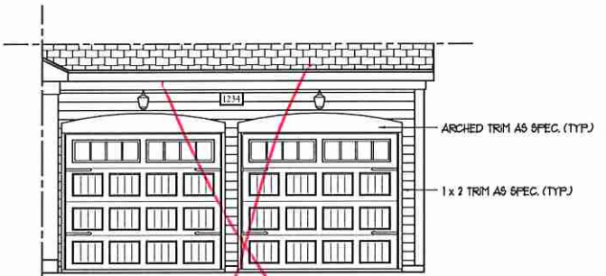
DOUBLE GARAGE DOOR OPTION SCALE: 1/4" = 1'-0"
