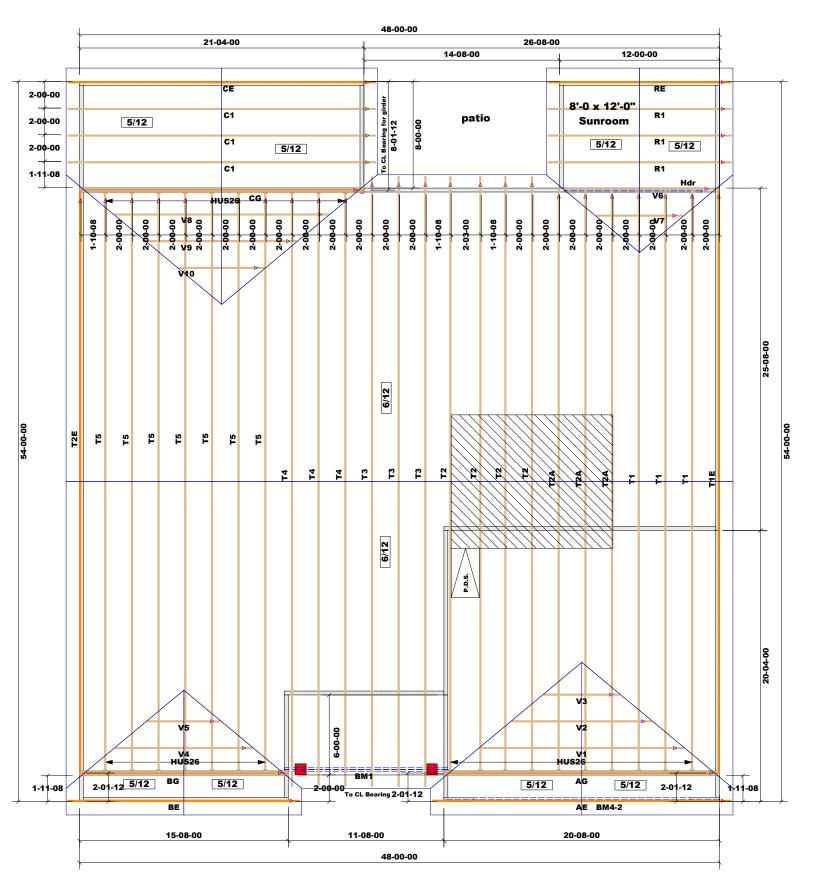
BM1 Dropped, carries Roof trusses T3 & T4 past front wall
