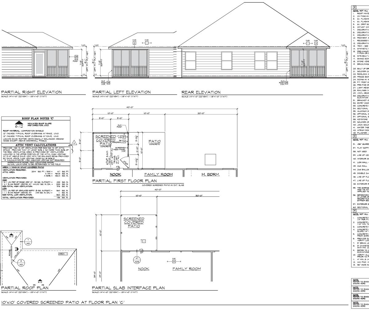
**ELEVATION NOTES** NOTE: NOT ALL KEY NOTES APPLY. ROOF MATERIAL - REFER TO ROOF NOTES 2X FASCIA/BARGE BOARD WITH FASCIA CAP G.I. FLASHING G.I. FLASHING & SADDLE/CRICKET 5. G.I. DRIP SCREED 6. 24"x24" CHIMNEY DECORATIVE VENT HOME DECORATIVE CORBEL DECORATIVE SHUTTERS IO. PEDIMENT. SEE ELEVATION FOR TYPE II. RECESSED ELEMENT
