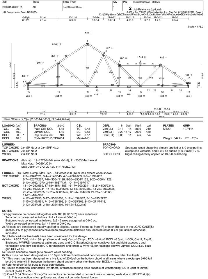
11) This truss is designed in accordance with the 2015 International Residential Code sections R502.11.1 and R802.10.2 and referenced standard ANSI/TPI 1.
