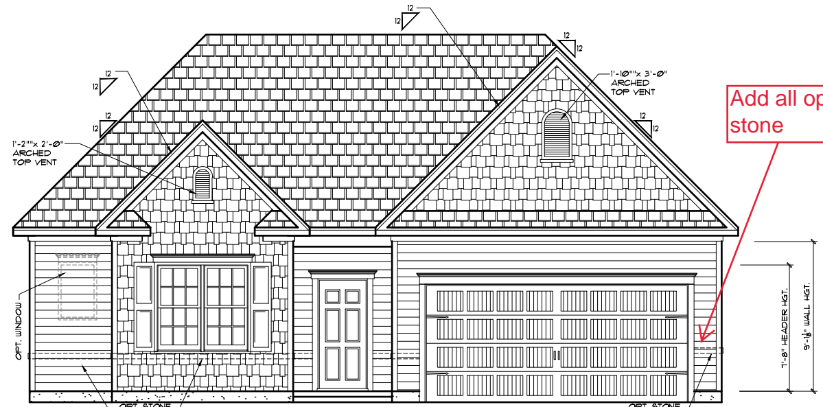
FRONT ELEVATION (WITHOUT GAME ROOM) 22x34 PRINTS SCALE: 1/4"=1'-0" 11x17 PRINTS SCALE: 1/8"=1'-0" CLASSIC
