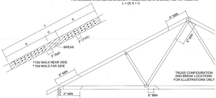
THE LOCATION OF THE BREAK MUST BE GREATER THAN OR EQUAL TO THE REQUIRED X DIMENSION FROM ANY PERIMETER BREAK OR HEEL JOINT AND A MINIMUM OF 6" FROM ANY INTERIOR JOINT (SEE SKETCH ABOVE)
