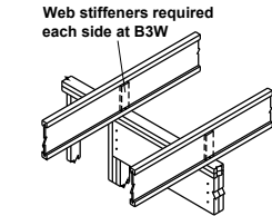
B3 B3W Blocking panels may be required with shear walls above or below (See detail B1)
