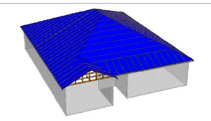
THE PURPOSE OF THIS DETAIL IS TO ILLUSTRATE HOW TO PROPERLY SPACE 24" O.C. ROOF TRUSSES TO ALLOW FOR A 25 1/2" OPENING FOR PULL DOWN ATTIC ACCESS
