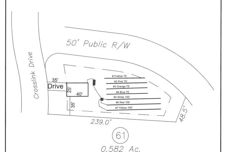
System: Gravity to D-Box Lines: 5-7, (300')
