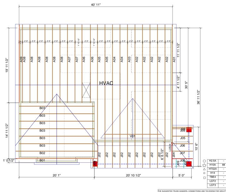
THE SUGGESTED TRUSS HANGERS, CONNECTIONS AND TIE-DOWNS FOR GRAVITY, JPLIFT AND LATERAL LOADS, MUST BE REVIEWED BY THE BUILDING DESIGNER OR REGINIERE OF RECORD. PER ANSI/TP1 1:2002, ALL 'TRUSS TO WALL' AND 'TRUSS TO BEAM' CONNECTIONS ARE THE RESPONSIBILITY OF THE BUILDING DESIGNER. ALL TRUSS TO TRUSS' CONNECTIONS ARE THE RESPONSIBILITY OF THE TRUSS DESIGNER/ MANUFACTURER
