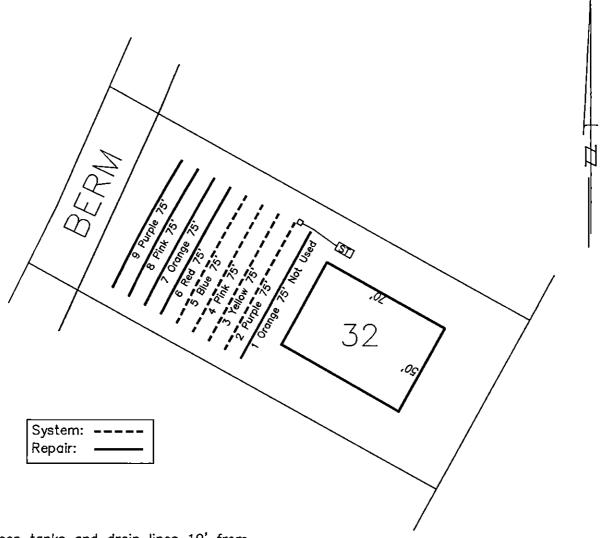
\*Keep tanks and drain lines 10' from property lines.
