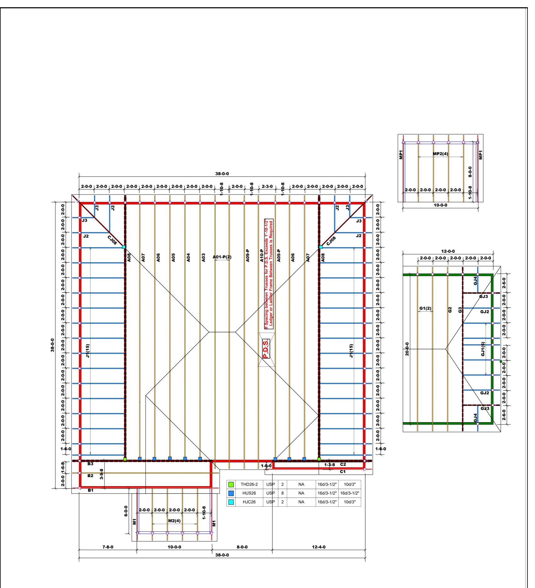
▲ = Indicates Left End of Truss (Reference Engineered Truss Drawing) Do NOT Erect Truss Backwards
