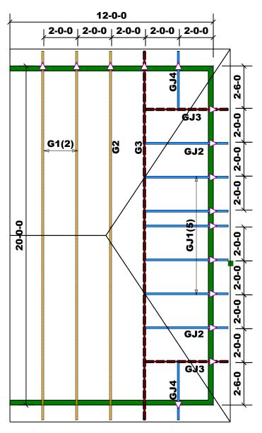
**Truss Placement Plan SCALE: NTS**
