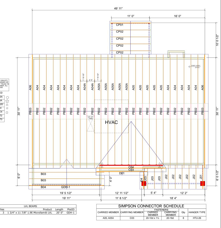
THE SUGGESTED TRUSS HANGERS, CONNECTIONS AND TIE-DOWNS FOR GRAVITY, UPLIET AND LATERAL LOADS, MUST BE REVIEWED BY THE BUILDING DESIGNER OR ENGINEER OF RECORD, PER ANSIFTID 1-2002, ALL "TRUSS TO BEAM" CONNECTIONS ARE THE RESPONSIBILITY OF THE BUILDING DESIGNER. ALL "TRUSS TO TRUSS" CONNECTIONS ARE THE RESPONSIBILITY OF THE TRUSS TO BEAM" CONNECTIONS ARE THE RESPONSIBILITY OF THE TRUSS DESIGNER/ MANUFACTURER
