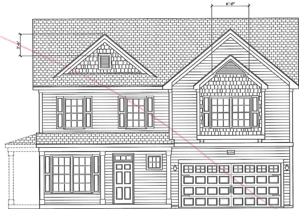
FRONT ELEVATION-A-1 SCALE: 1/4" = 1'-0"
