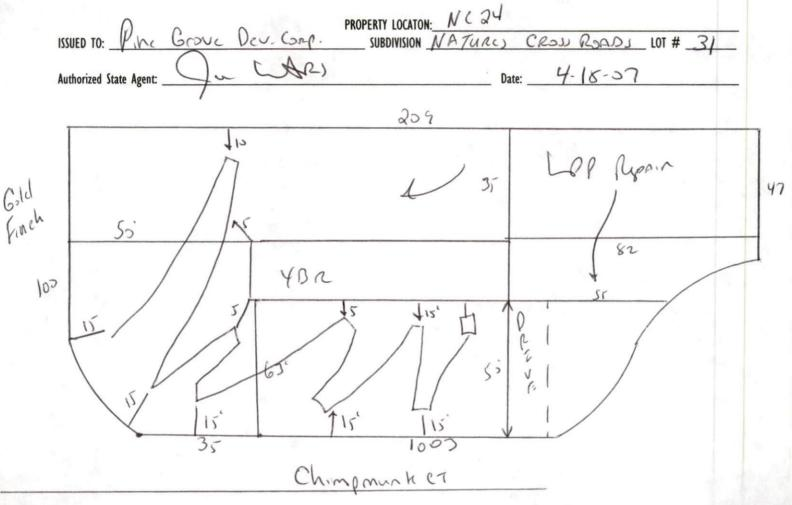
STUB Out Plumbing shallow, at Ground level or hisher, where shown Mpintain All set Breks keep drain Line, Is from Top of Road Dth Intal 1x240 At 18 to 24" Deep. There is some Road spoil Fill in the Front of The Lot keep drain Lines 6" Below Fill.
