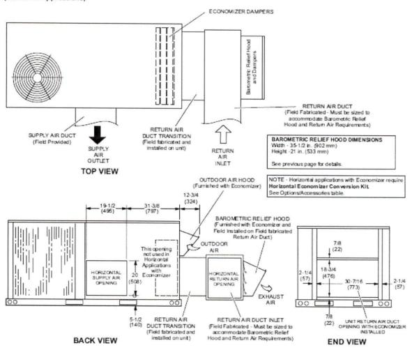
NOTE - Return Air Duct and Transition must be supported.
