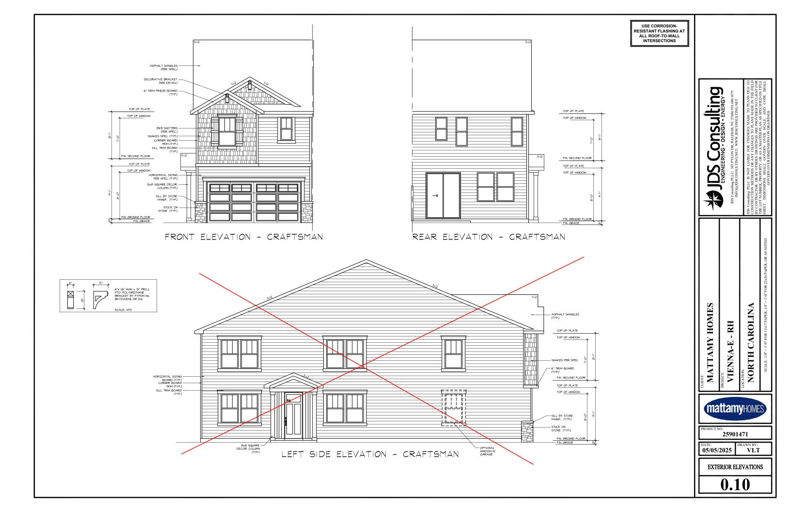
USE CORROSION-RESISTANT FLASHING AT ALL ROOF-TO-WALL INTERSECTIONS
