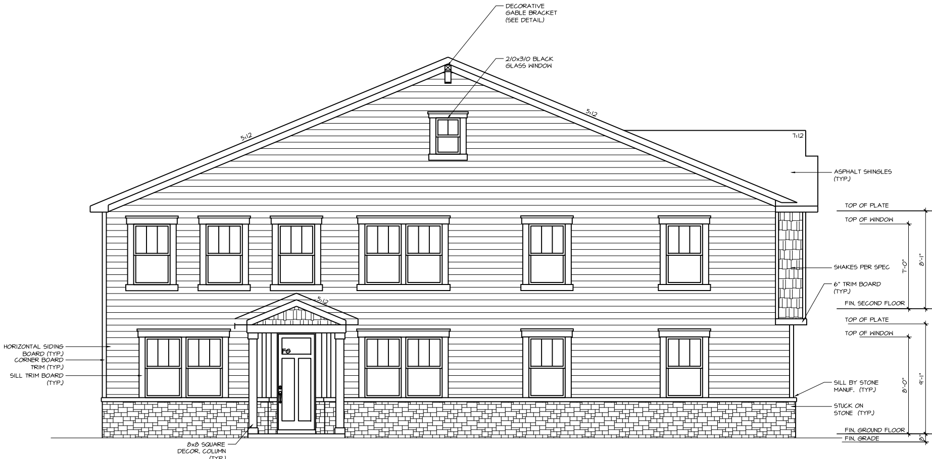
LEFT SIDE ELEVATION - CRAFTSMAN UPGRADED SIDE ELEVATION
