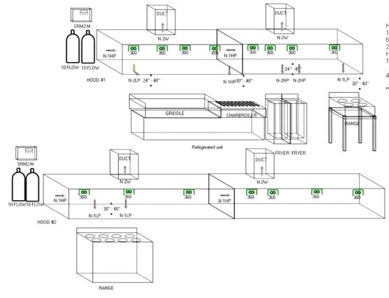
Hood 1- 16'L x 4'W. 2 ducts @ 16" x 16. Buckeye BFR-10/10 fire system. 1 tank covers appliances using 8 flows. 1 tank covers plenum and ducts using 6 flows. 60" x 22" griddle, 36" x 22" radiant chargrill, Double vat fryer (vats 13" x 16" each) 24" x 24" 4 burner stove.
