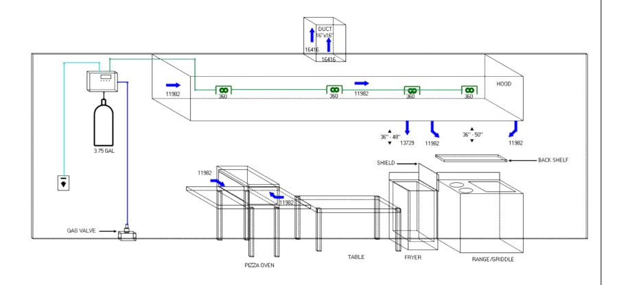
This is an Amerex kitchen fire suppression system model KP 375, which has a maxmimum flow point of 11.
