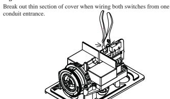
Fig. 5 Switch Terminal Connections Clamping Plate Terminal
