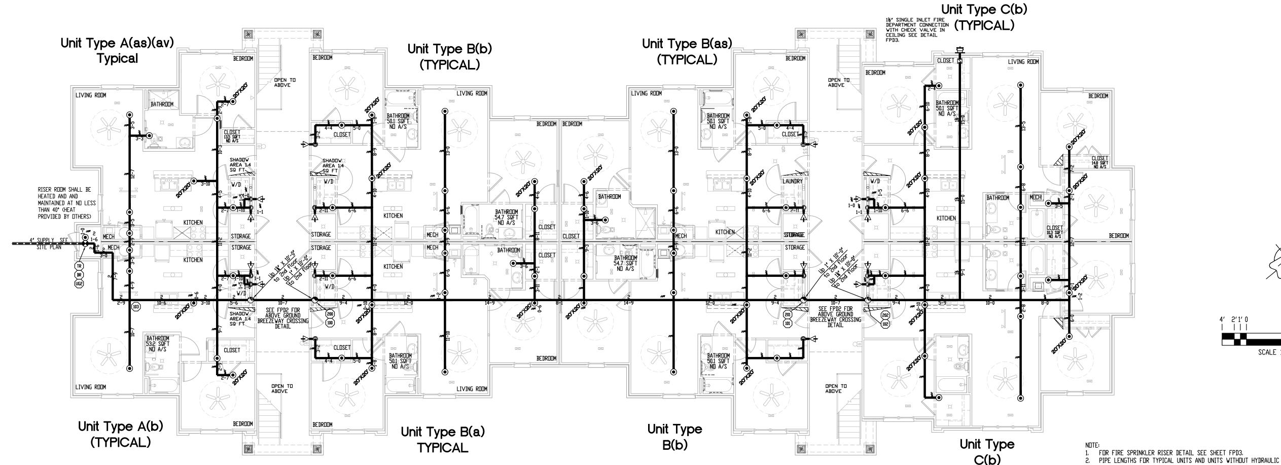
BUILDING 200 - 1ST FLOOR FIRE SPRINKLER LAYOUT
