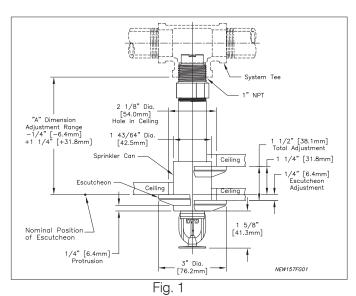
Note: The sprinkler can protrudes ¼" when escutcheon is in nominal position. Escutcheon adjustment provides -1¼" (-6mm) to +11¼" (+32mm) "A" dimension adjustment range.
